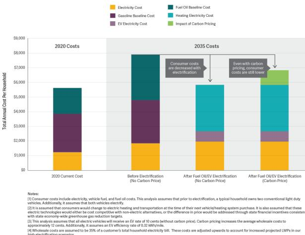
Figure ES-2: Estimated Average Annual Consumer Energy Costs for Households that Adopt Electric Vehicles and Convert Home Heating System from Fuel Oil to Electric Heat Pumps
